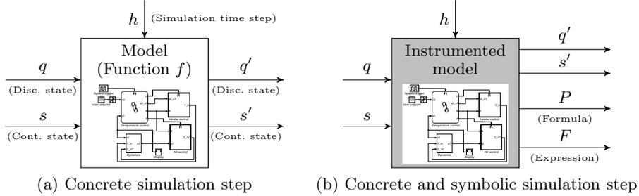
**Fig. 1.** Single-step concrete and symbolic simulation semantics of SL/SF models
