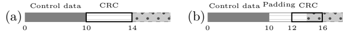
■ Figure 1 Mis-interpretation of a MAC ACK frame by an Atheros receiver: (a) Layout of the incoming ACK frame and (b) The type-incompatible layout computed by the receiver
